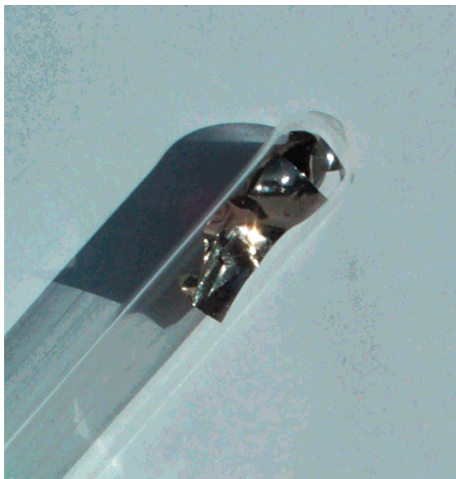
Figure 1. Picture of a trans -polyacetylene sample provided by Professor Alan Heeger, October 2001 (picture courtesy of Demetrio Filho).
